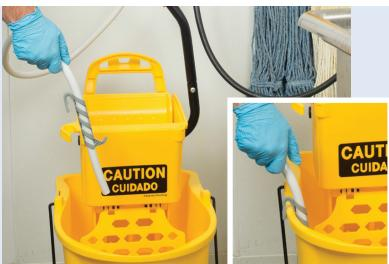
Insert and clip discharge tube into mop bucket or automatic scrubber tank using hose hanger.
